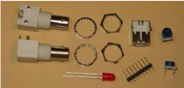
BNC connectors, washers, nuts USB connector Trimmer resistors LED Backpanel 8-pin connector
