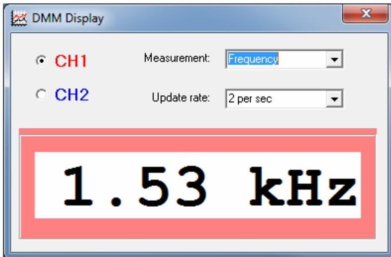
While the automated measurement panel is convenient, sometimes you may want to observe only a specific value. This could be e.g. to trim the frequency or the amplitude of an oscillator. Chances are you do this at some distance from the screen so it is important that the display is large enough to be observable without being right in front of the computer.
