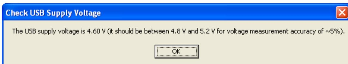
For early versions of the scope (firmware prior to V2.1) you will also be given the option to use the measured voltage to calibrate the vertical scale . this will make the display as accurate as for V2.1 and later revisions even when the supply voltage is not exactly 5V. Simply choose **Yes** when asked if you want to apply the correction:
