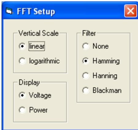
Checking the **FFT** option will change the display to frequency domain: The oscilloscope performs a real-time FFT (Fast Fourier Transform) on each captured record. This is a highly useful mode to analyze periodic signals or to find small periodic components (e.g. periodic noise from the power line) hidden in the main signal. It is much easier to see an isolated 60 Hz component (spectral line) in a frequency plot than it is to see it among all the random noise riding on the signal.
