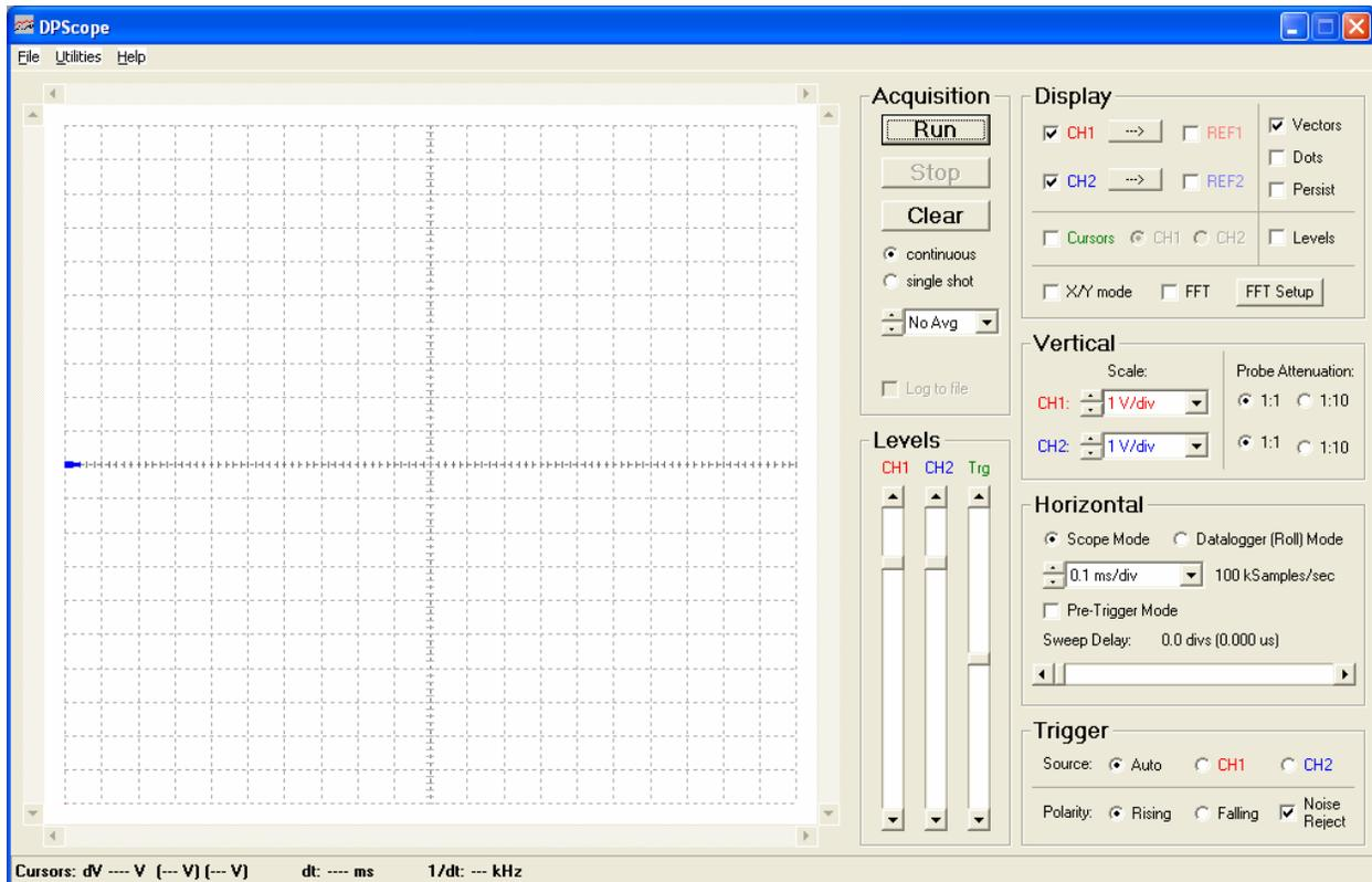
The left side of the display is taken up by the waveform display. On the right side you can see that the controls are grouped in several functional blocks (we will explain each of them in more detail later):
